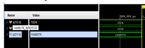
Fig: 6.8. 16-Bit Proposed Wallace tree multiplier Simulation Result.
