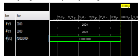
Fig: 6.7. 8-Bit Proposed Wallace tree multiplier Simulation Result
