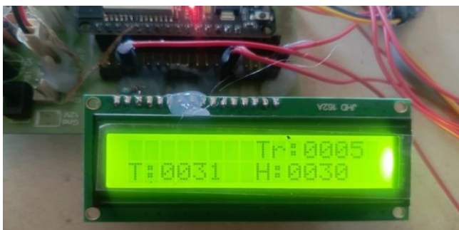
Fig 5: Display Showing "Temperature, Humidity, Turbidity"
