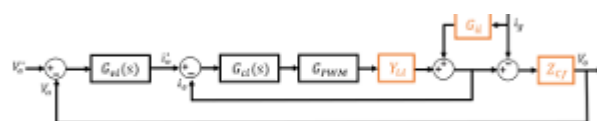
FIGURE 2. Block diagram of the voltage-controlled inverter. ZLl(s) and ZCf(s) represent the impedance of the filter inductor and a capacitor with a damping resistor.
