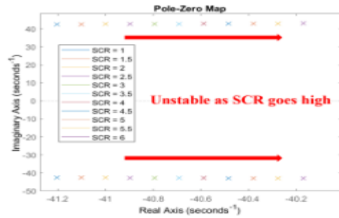
FIGURE 4. Grid-forming (GFM) inverter plant model pole considering the short-circuit ratio (SCR).
