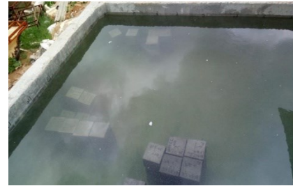
Curing of specimens
