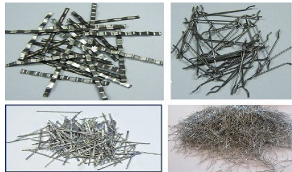
Steel fibre of (a) anchor steel fibre (b) hooked end steel fibre (c) reinforced steel fibre (d) recycled steel fibre
