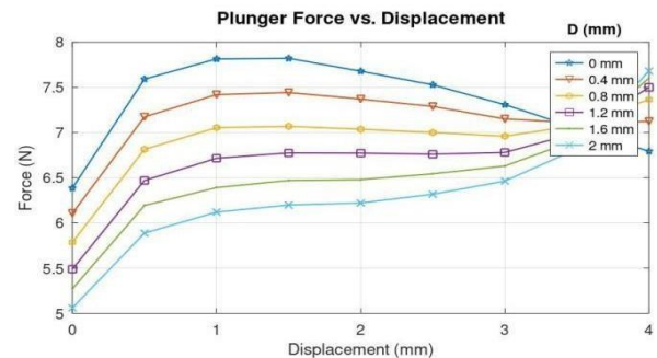
Figure 14 Plunger Force vs. Plunger Displacement characteristics for various positions of D in the second iteration
