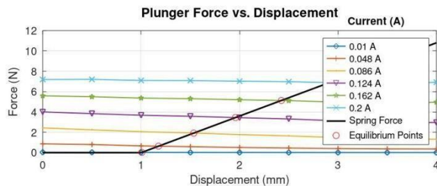
Figure 25 Force vs Displacement characteristics of the Proportional Solenoid and the restraining spring (1 mm offset)
