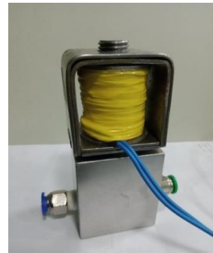
Figure 21 The developed proportional solenoid valve for flow control
