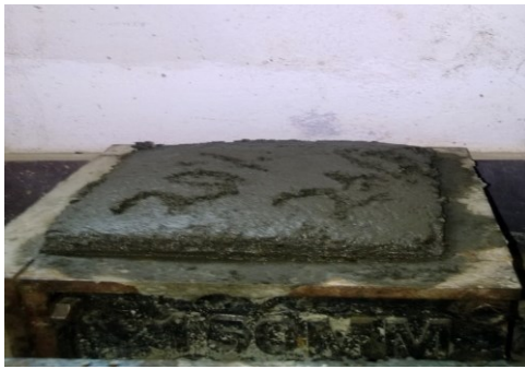
Fig: 10. Expansions of Concrete Cubes
