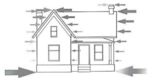
Lateral loads acting on the building
