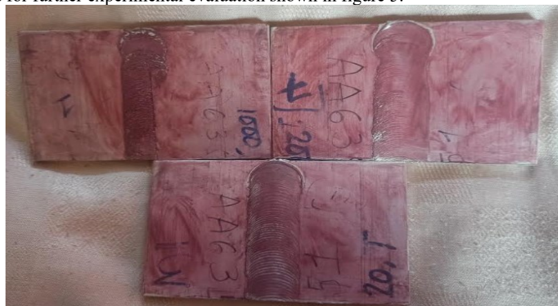
Figure 5 Dip coated AA6351 welded samples
