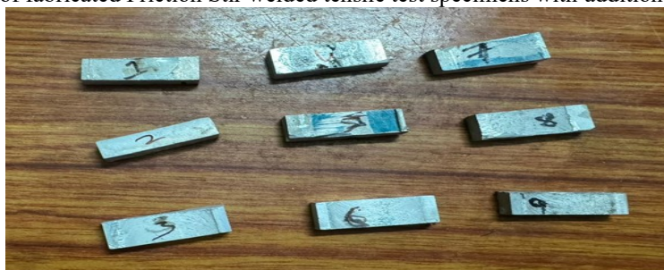
Figure 10 Photograph of fabricated Friction Stir welded hardens test specimens with addition of \text{AgNO}_3 Nano coated
