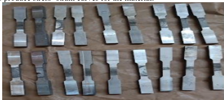
Figure 3: Photograph of fabricated Friction Stir welded tensile test specimens
