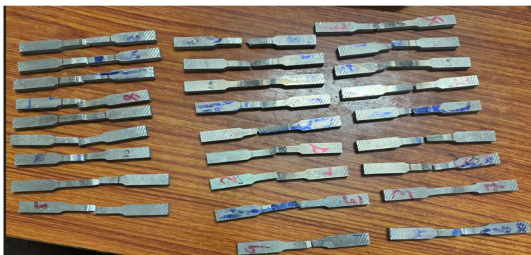
Figure 9: Photograph of fabricated Friction Stir welded tensile test specimens with addition of \text{AgNO}_3 Nano coated
