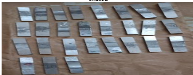
Figure 11 Photograph of fabricated Friction Stir welded Microscopic test specimens (SEM) with addition of \text{AgNO}_3 Nano coated
