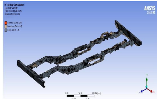
Fig 9. Topology Optimization Result Showing Elemental Density Distribution for Titanium Alloy Chassis
