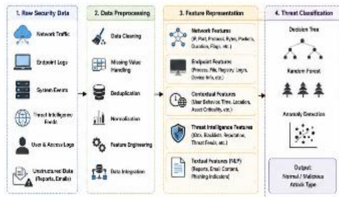
Fig. 2. Security Data Processing and Threat Classification Pipeline
