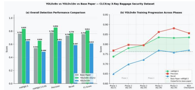
Fig. 2. Left: overall metric comparison across all three models on the CLCXray test split. Right: YOLOv8n mAP@0.5, precision, and recall convergence across training phases. The dashed horizontal line marks the base paper mAP@0.5 of 0.762; the shaded green region highlights epochs where the proposed model surpasses this threshold.
