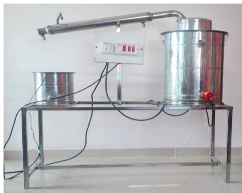
Fig. 1 Experimental Setup of Steam Distillation Unit
