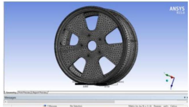
Figure 3. Finite Element Mesh of the Wheel Rim
