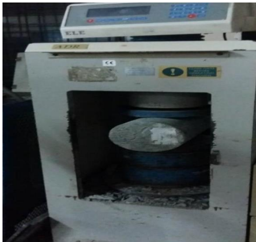
Fig. 2.10. Split tensile strength Test
