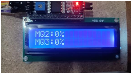
Fig. 4 Show the value of the MQ sensor on the LCD.
