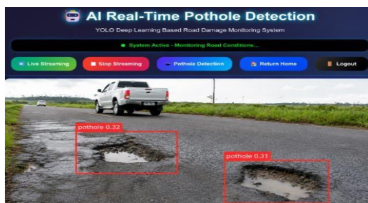
Figure 6: Live Video Streaming and Real-Time Road Damage Detection
