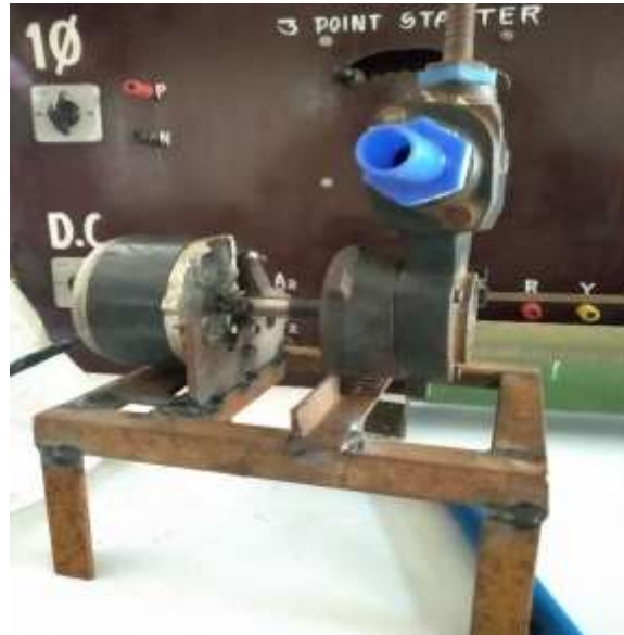
Fig 7. Dc motor-pump set
