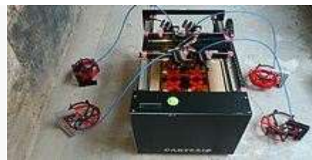
Fig 10. CartesioLDMP mass production 3Dprinter
