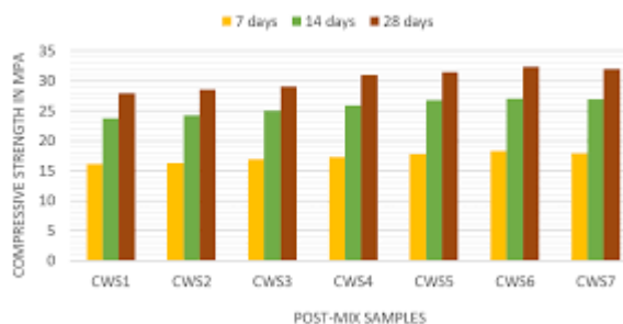
fig. 1. compressive strength development at 7, 14, 28, and 56 days for all nano-silica dosages.
