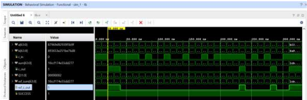
Fig 7 Simulation waveform of Hybrid Adder (CLA (32-bit) + KSA (32-bit))
