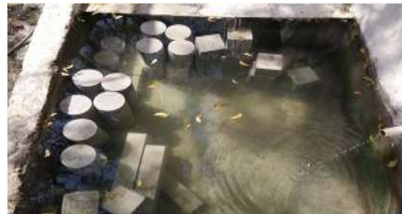
Test specimens kept for curing
