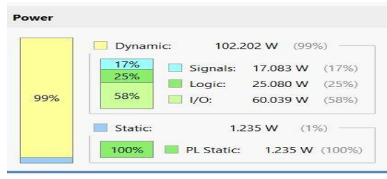
Fig 3: Existing Power for N=32
