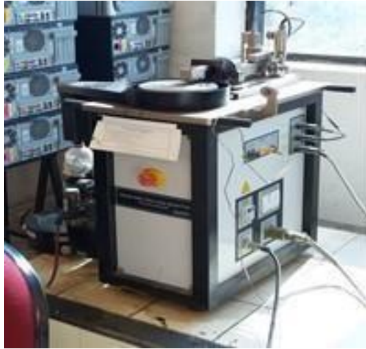
Fig. 2. Pin on Disc Apparatus
