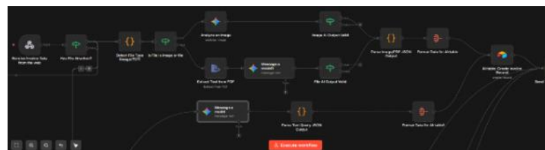
Fig. 3. Agent Routing Workflow (GST, TAX, Accounting)- n8n multi-agent routing workflow illustrating the Text Classifier node, intent-based dispatch to TAX, GST, and Accounting agents, and their respective memory and tool integrations.
