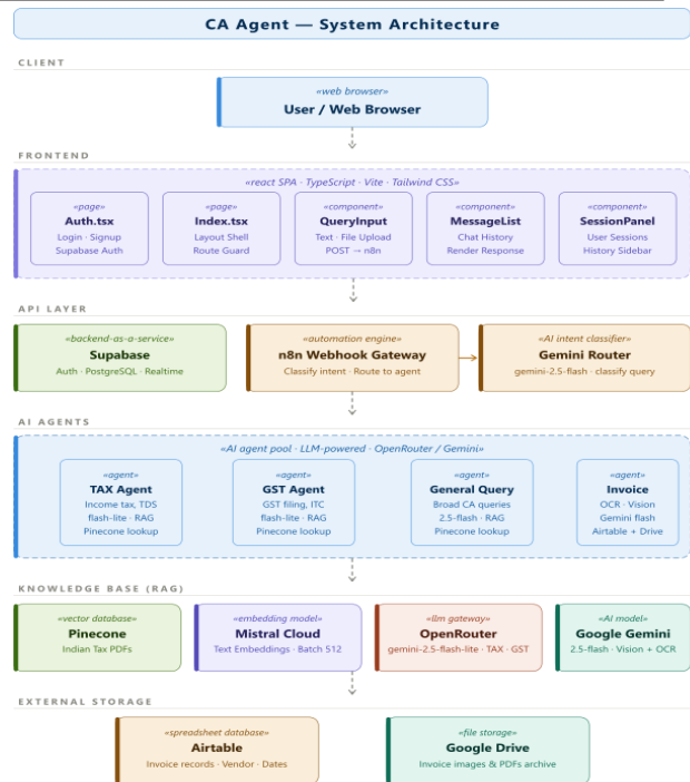
Flow: User query → React UI → n8n webhook → Gemini classifier → Agent selected → RAG (Pinecone+Mistral) → JSON response → Supabase saved → UI renders
