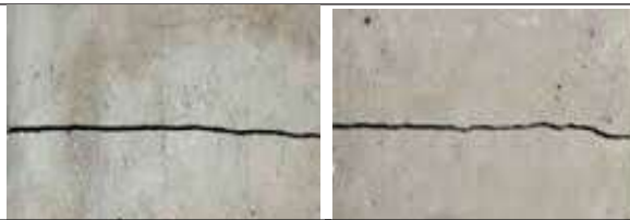
The fig shows the crack made in the Concrete Cube made up of Bacillus Pasteurii
