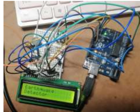
Fig.1 Embedded Hardware Kit for Structural Monitoring
