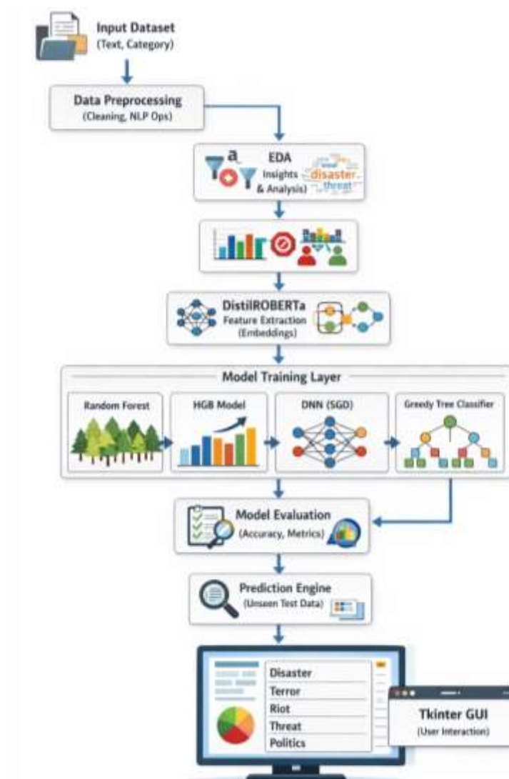
Figure 2: Proposed system architecture
