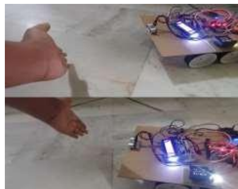
Figure 4 a: Cart following the customer using ultrasonic sensors
