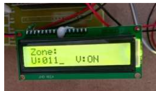
Figure 7. LCD Display Showing Vehicle Speed Control Status
