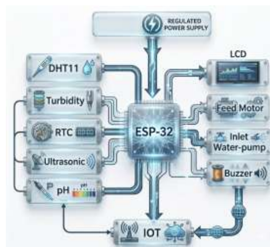
Figure 1. Block Diagram of ESP32-Based IoT Fish Farming Monitoring and Automation System.
