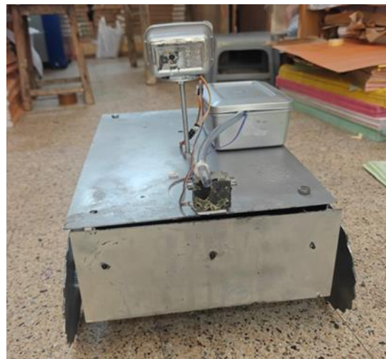
Fig: The finalized Fire-Bot Pro prototype. The image highlights the heavy-duty serrated metal wheels designed for traction and the specialized metal enclosures that protect the ESP32-CAM and control circuitry from direct heat exposure.
