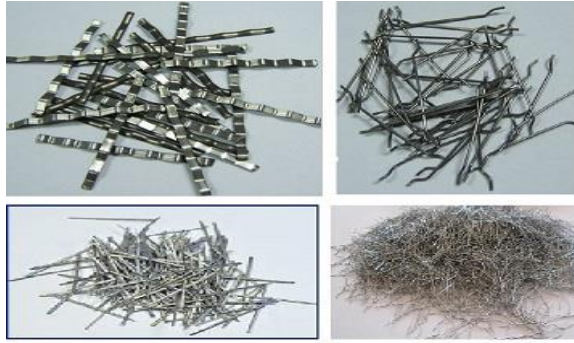
Steel fibre of (a) anchor steel fibre (b) hooked end steel fibre (c) reinforced steel fibre (d) recycled steel fibre
