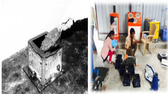
Filling the mould (for 150 mm cube 3 equal layers)
