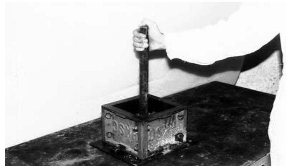
Compacting the concrete in the cube mould (For 150 mm cube at least 35 tamps per layer)
