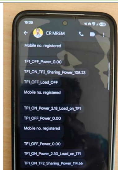
Fig.4: GSM-based fault and load status alerts on registered mobile device
