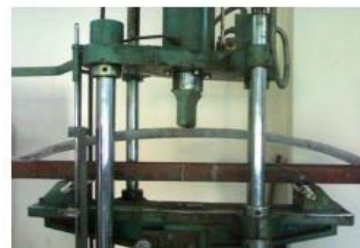
Fig. 6 Load applying on GFRP Leaf spring
