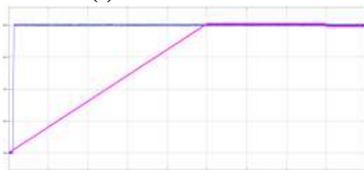
FIGURE 22. Transient result for suddenly increasing the output power from the solar cell array.
