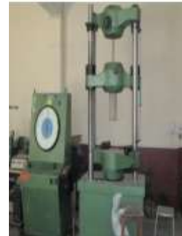
Fig 10: Testing of bond strength of concrete
