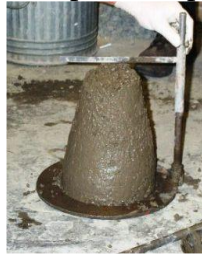
Fig4.2. Measuring Slump Fall
