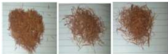
Fig 4: Coconut fibre of 10mm, 15mm & 20mm Length
