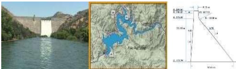
Figure 1. Geometric conditions of Pine Flat Dam (2)
