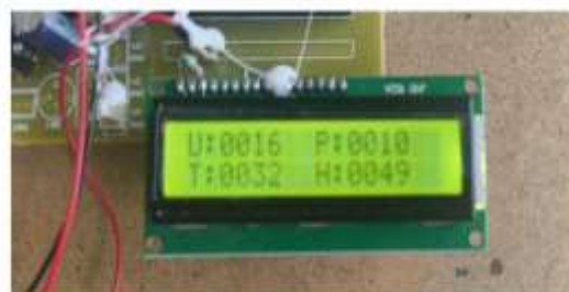
Fig. 4: Real-Time Sensor Data Display on 16x2 LCD in IoT-Based Aquaculture Monitoring System.
