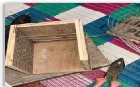
Fig: Wooden Mould With 2mm Optical Fibers
