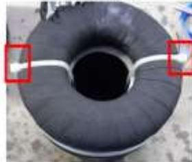
FIGURE 10(a). Secondary coil with cable tie
