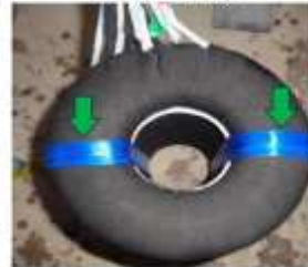
FIGURE 10(b). Secondary coil with ribbon
