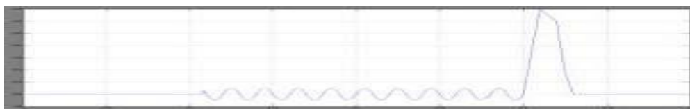
Fig.3.11 Short-circuiting PV panels dc-link voltage when applying a 60% SLG voltage sag at MV side of the transformer
